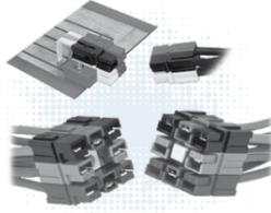
PP15-45 series are the smallest Powerpole® housings. They can be used for wire-to-wire or wire-to-board applications. Wire sizes from #20 AWG (0.75 mm<sup>2</sup>) to #10 (6 mm<sup>2</sup>) offer power capabilities up to 55 amps per pole. Finger proof housings and the ability to incorporate first-mate last-break ground connectors enhance the capabilities of this Powerpole® series.
