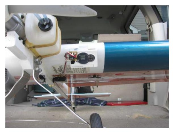
The camera is velcro'ed and taped onto the wing. The square in the middle of the camera is the mode display. On the right is the lens and in the upper left is the servo interface circuit. The camera will hold up to 60 "high resolution" pictures – for the definition of high resolution, I refer you to the title of this article. The camera is triggered by a switch on my transmitter and can take a picture about every three seconds. Again remember, cheapest digital camera money can buy.
