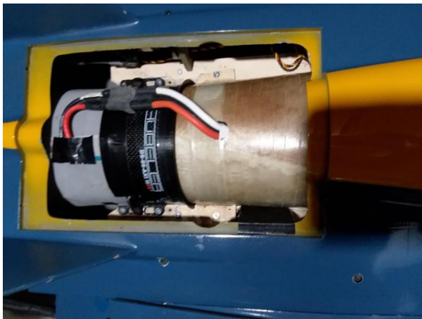
CLOSED DUCTING WITH BELL MOUTH as a transition
