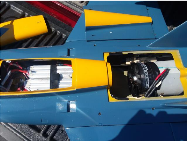
OPEN DUCTING WITH BELL MOUTH
