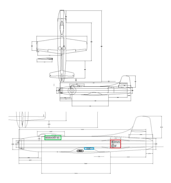
The 3 sections of the fuselage are temporarily glued together and the hatch has been cut out for the FMS 80mm EDF unit. The forward section, from the nose to the rear of the canopy, will have a 1/64<sup>th</sup> thick ply liner for the battery area support. This was because to get the 6S battery to fit will require removal of all the foam the in that area.
