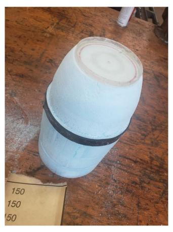
Poster board template for section 1 (nose). I modified my Dremel scroll saw to be a hotwire jigsaw. A series of 2" thick disk will be stacked and glued together. Once together, I can start the fun part, making blue dust.
