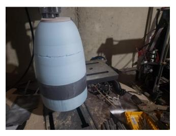
With the initial hand sanding done time to temporarily glue ends on to mount it to the drill press for more sanding. The center, for ducting will have to be removed. I haven't decided if I will cut it in half or drill a starter hole for the hotwire.
