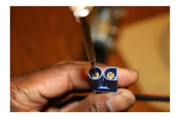
If you are using this or any connectors you should inspect them periodically. This is really important if you have a ESC with a built-in BEC to power the RX and servos
