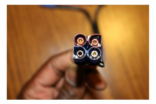
The adaptor on the left is what I made to minimize wire length and make it more compact, it is soldered or butt spliced to the ESC also eliminating the  $3^{rd}$  connector. Back to Bill's F/A-18, when a
