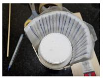
Once the shape has been achieved by rolling over a rounded surface. It can be mounted to the model and tape can be removed. For thinner Depron I have had luck with rolling it over a rounded table edge or a bottle/tin can with no other prep needed, unless the radius is small. If the radius is small, then use the steps above.
