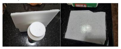
Apply the packing tape to the planned outside of the sheet. This is to prevent breaking, cracking and excessive creases.
