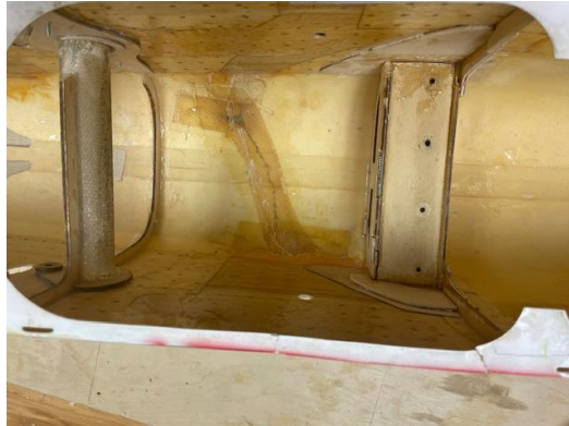
Photo 7: Bottom of fuselage fiberglass repair.
