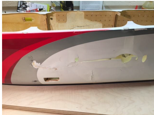
Photo 2: Left skin damage and right damage core removed.
