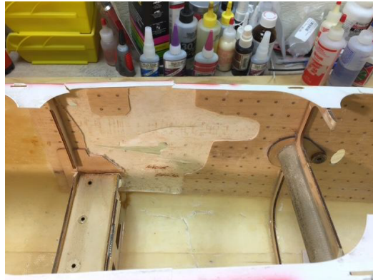
Photo 4: Minimum of damaged core and inner skin removed.
