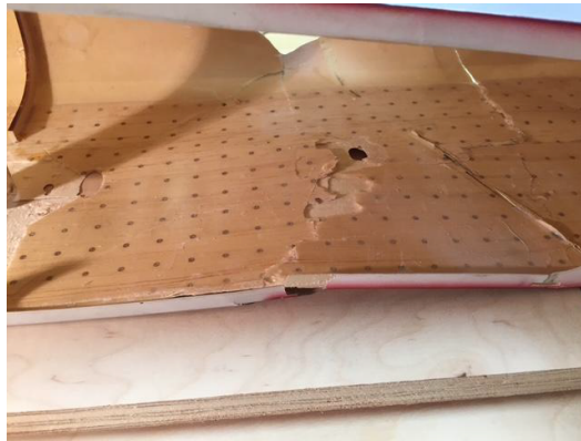
Photo 1: Fuselage side balsa core damage. This fuselage side skin is a sandwich structure with an outer fiberglass skin, a balsa core and a thin inner skin.
