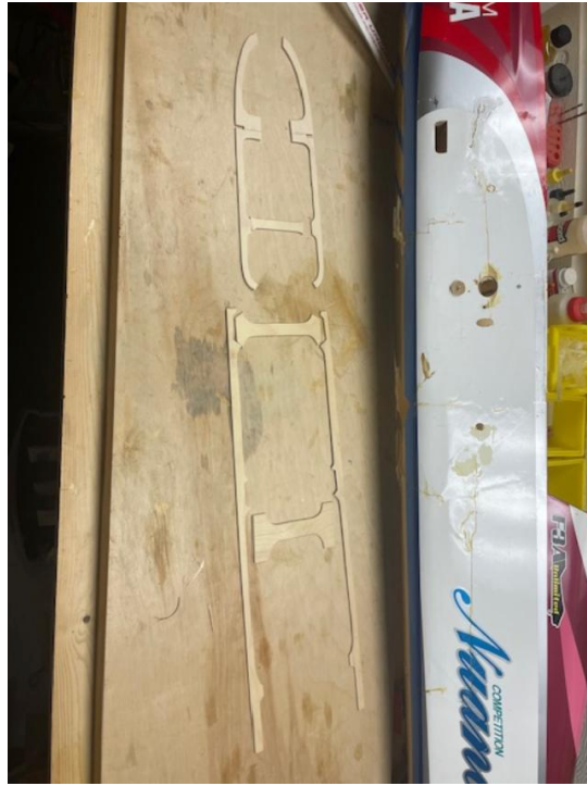
Photo 9: Canopy sill parts ready. The airplane did not have these originally, but with the monocoque damage these are needed for stiffness and to straighten the sides.
